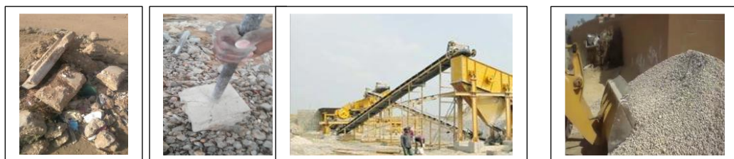
Figure 1: The aggregates recycling process
